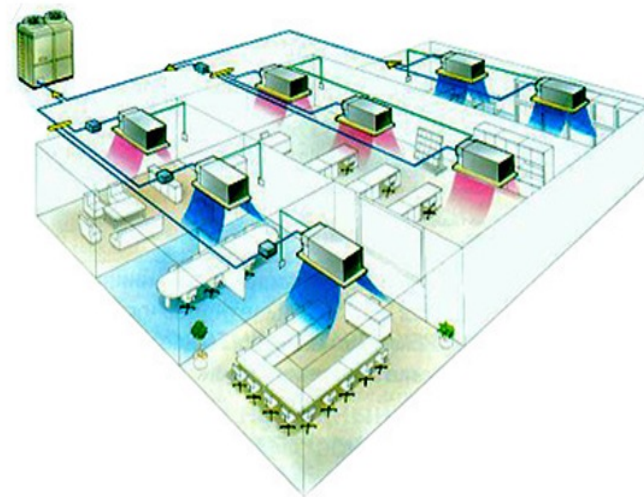
Figure 5. A typical VRF application
