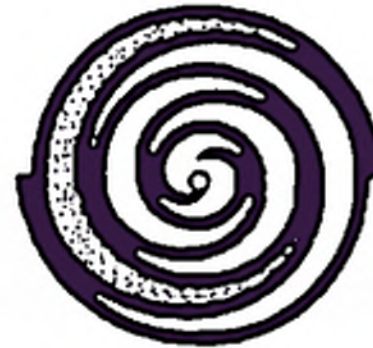
(b) The pocket is sealed off and compression starts
