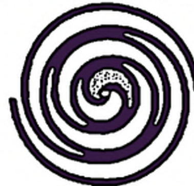
(b) The pocket is sealed off and compression starts
